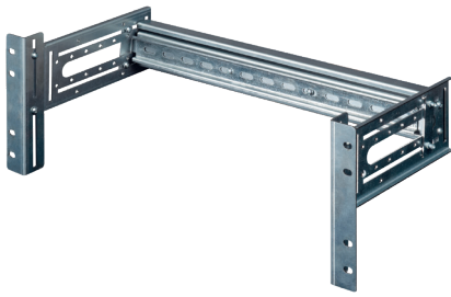
4U Mounting 19" ears, DIN rail set to back, 19" rails adjusted to top elevation.
